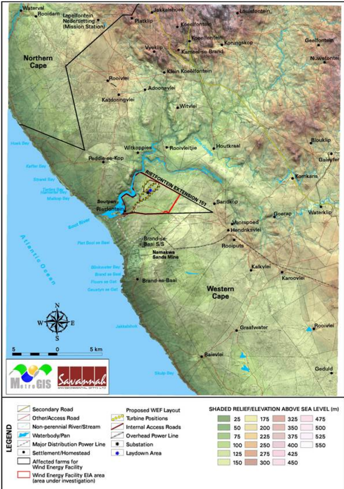
Map 1: Locality map and proposed layout of the proposed Exxaro West Coast WEF showing the provisional placement of infrastructure and shaded relief (topography and elevation above sea level)
