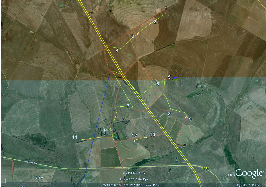
Figure 1: Proposed infrastructure layout for the northern area (north of R315). Brown lines are internal access roads, green lines are cable trenches, blue lines are internal, above ground electrical connections between the three substations, and white marks and numbers are turbine positions and numbers.
