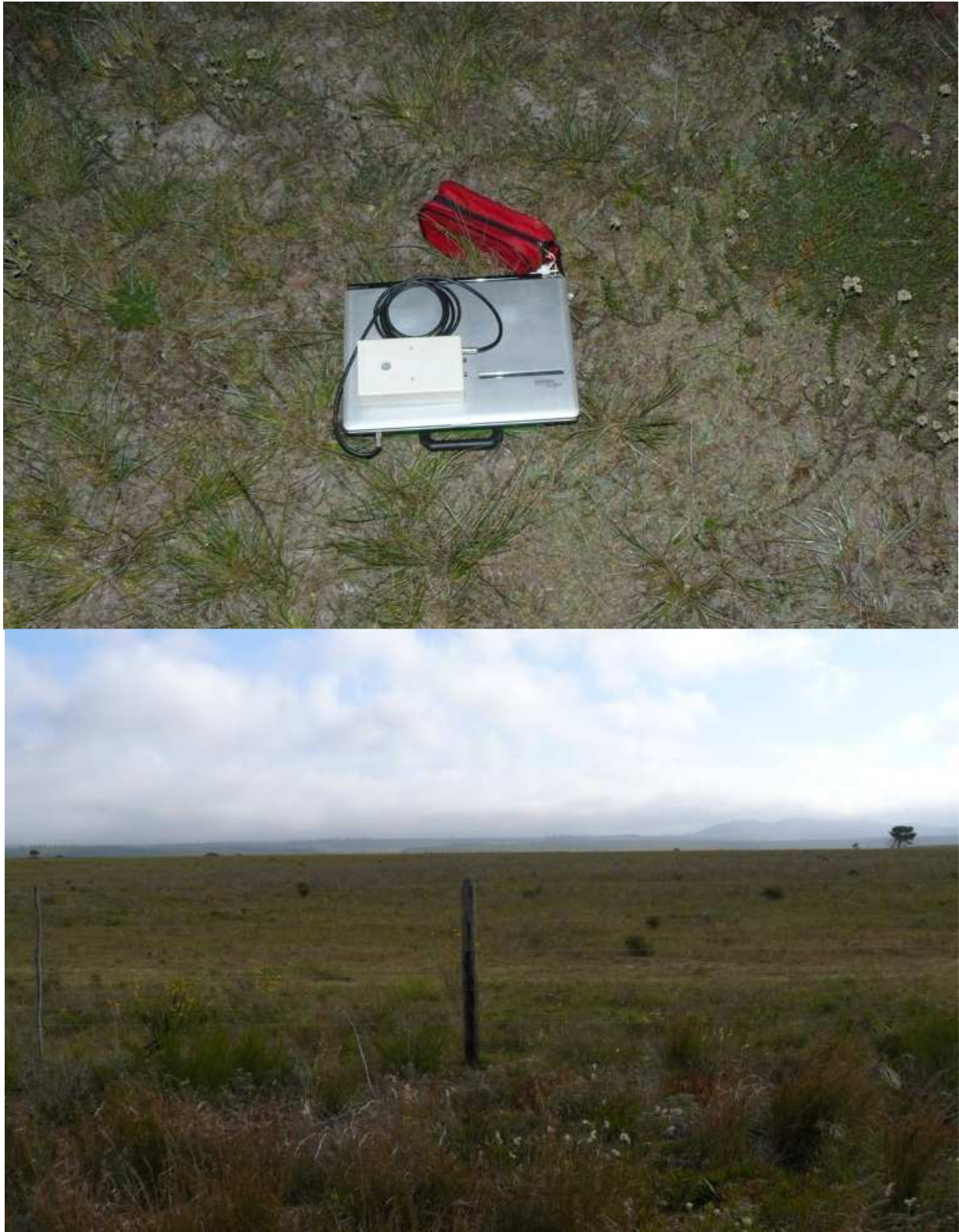
Figure 6: (top) The time expansion type bat detector (BD2) set up with a field laptop and external long life battery to passively record bat echolocation calls; (bottom) the flat open areas of the site where the proposed turbines are to be located, such open terrains unsuitable for mist nets.
