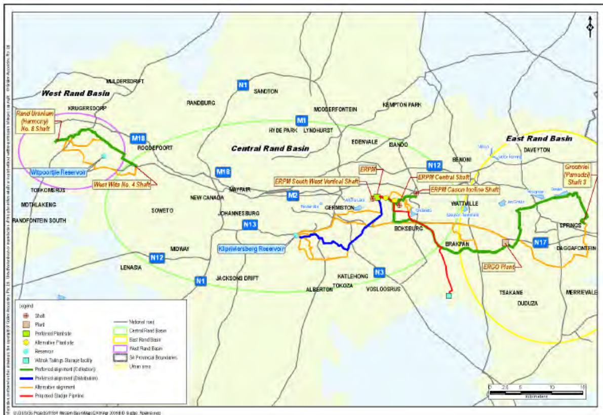
Figure 3: Preferred and alternative collection, distribution and sludge pipeline routes for the Mine Water Reclamation Project
