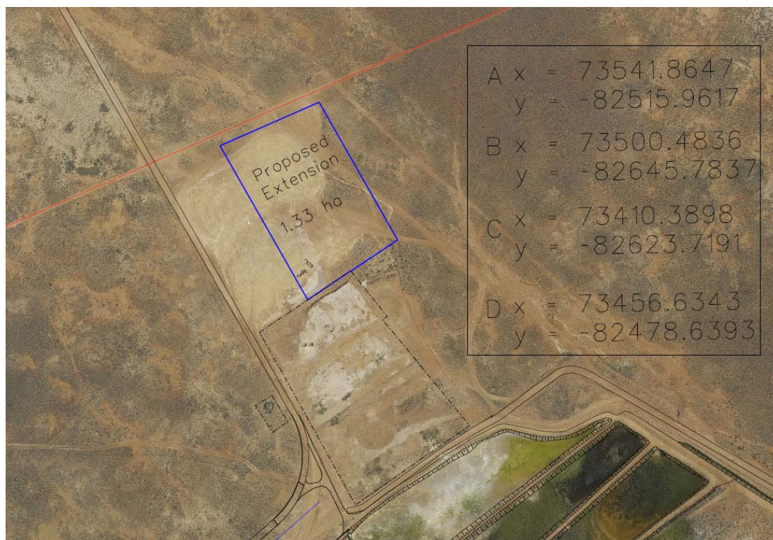
Figure 2: Detail showing proposed landfill extension area.
