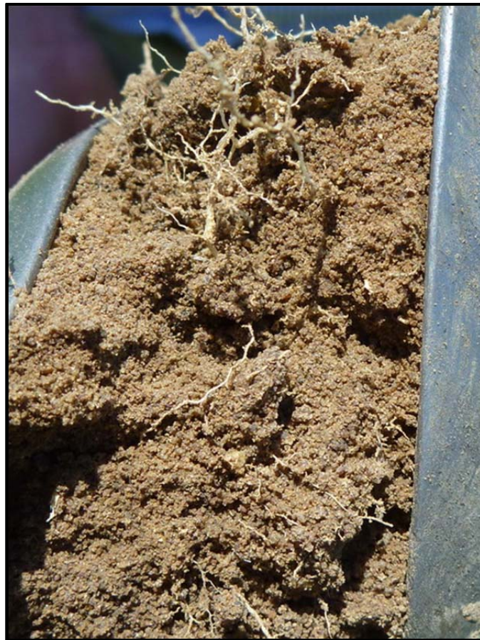
Figure 6 The orthic A-horizon that overlies the subsoil horizons of the Tukulu soil form is bleached in colour and exhibit a sand clay loam texture
