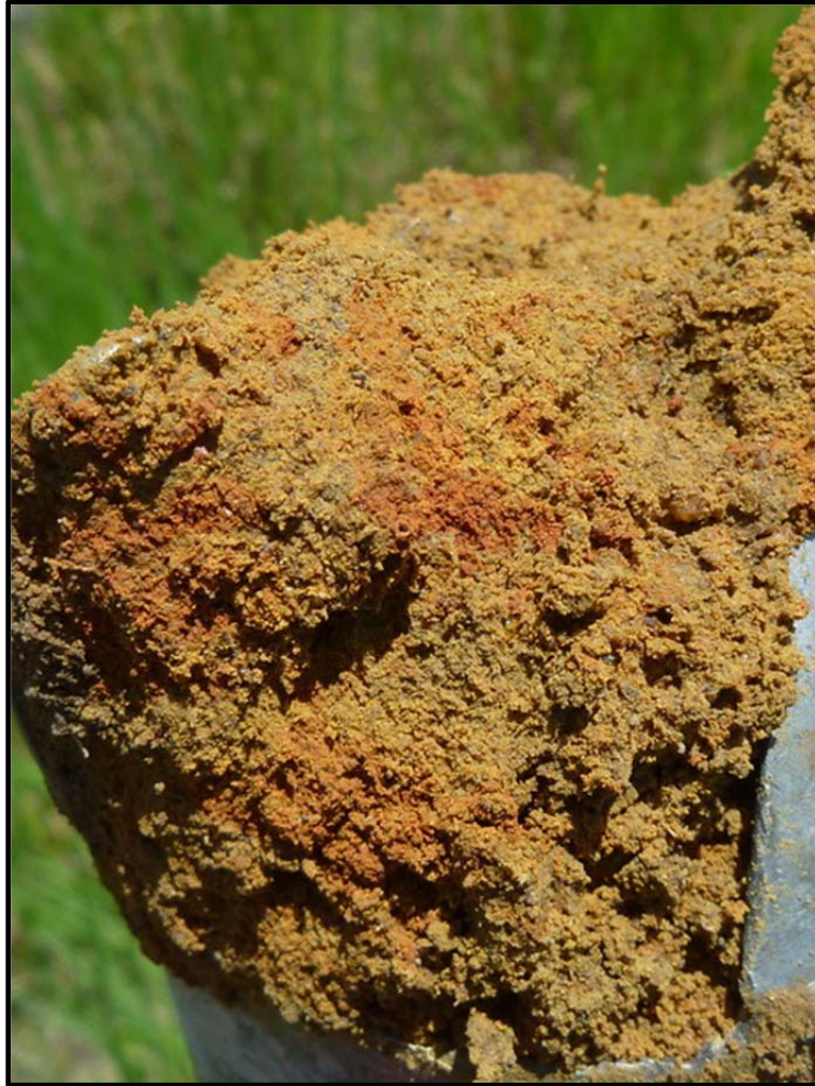
Figure 9 Signs of wetness is ascribed to conditions of reduction that leads to iron movement and the occurrence of red, yellow and black mottles and/or bleached colouration
