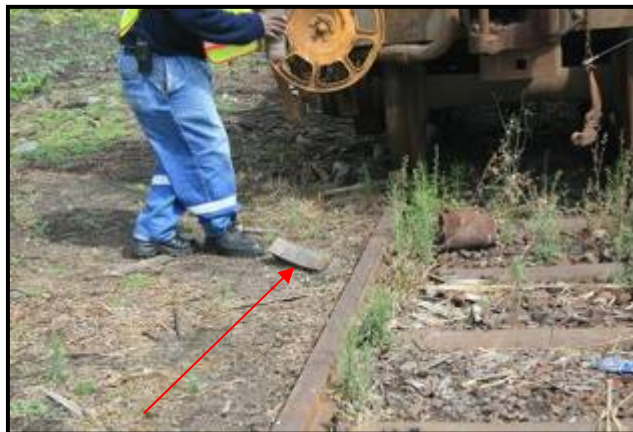
Figure 5: Nelspruit – Asbestos Containing Brake Blocks
