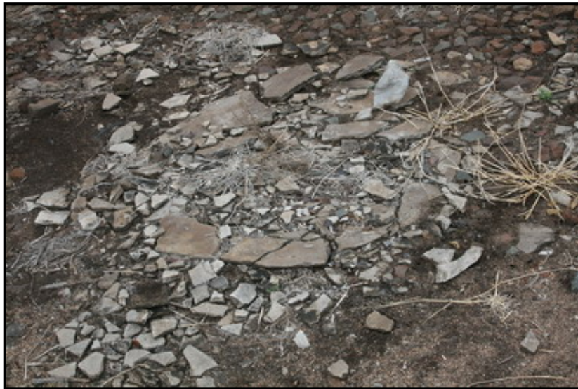
Figure 1: Nelspruit – Mixed asbestos waste
