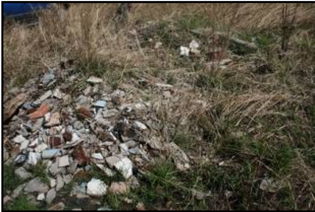
Figure 14: Barberton – Mixed Asbestos Waste
