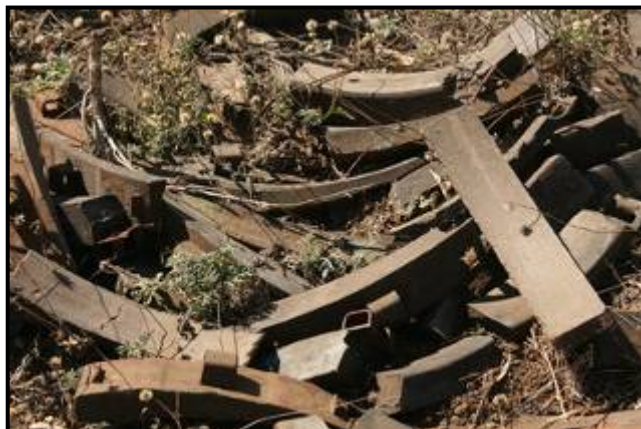
Figure 8: Komatiepoort – Asbestos Containing Brake Blocks
