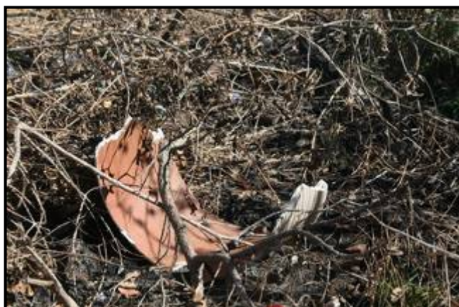
Figure 12: Barberton – Broken Asbestos Cement Waste
