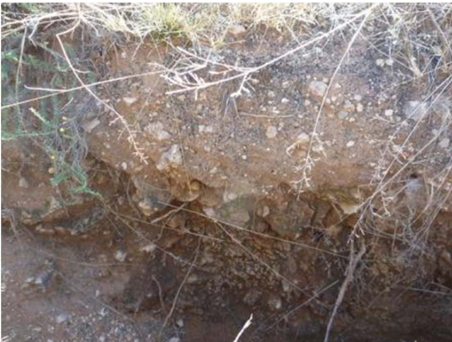
Figure 14 Exposed profile with lime pebbles in the matrix in the lime dominated area
